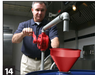
14 Attach hose or place funnel in oil disposal container opening. Turn pump handle toward spout to pump out oil. (No flow. See troubleshooting section.)
