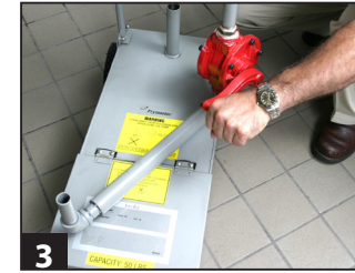
3 With the pump inverted turn the handle clockwise 3-4 turns stopping before oil pumps out of the spout.
