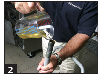
2 Invert pump and pour 1 cup of clean cooking oil into the pipe.
