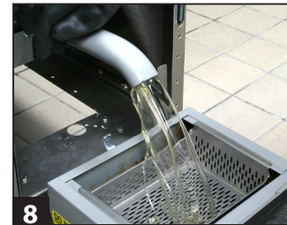
8 Open drain valve; drain oil into SDU; close drain valve. Remove and store drain extension.
