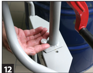
12 Release locking pin on pump head.
