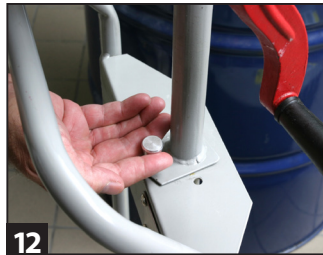
12 Release locking pin on pump head.
