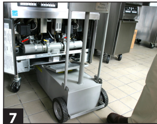
7 Slide SDU under filter drain down-spout.
