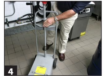
4 Reseat the pump and pipe unit on the SDU.
