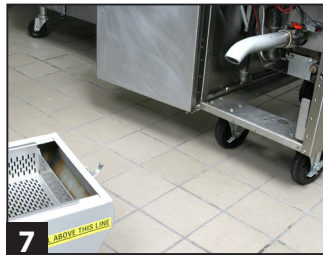
7 Position SDU under drain extension.
