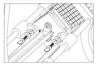
3) Attach cutter block to base and secure with washers and wing nuts.
