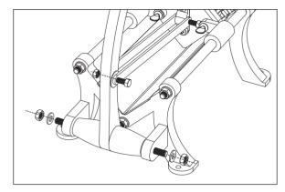
2) Attach push block in the center of base and secure with thumb screws.
