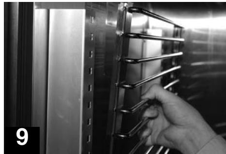
Type Kit #2 (Rod Style Tray Slide)
