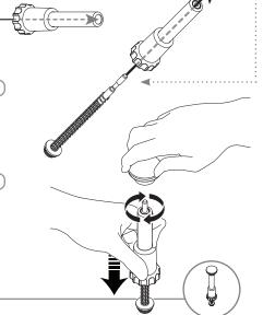
**INSTALL LARGE O-RING** into valve body. Apply food equipment lubricant on o-ring.
