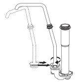
onto valve body. Rotate discharge tube clockwise and press down firmly to secure into slots on valve body.
