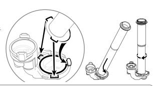
**INSTALL MEDIUM O-RING** onto discharge tube.
