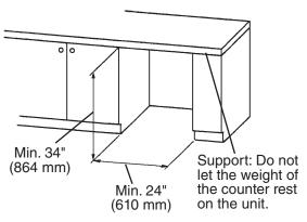
There must be at least 1" (3 cm) clearance between the top of the unit and the bottom of the counter.
