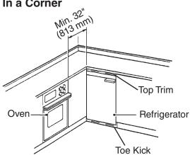
There must be at least 1" (3 cm) clearance between the top of the unit and the bottom of the counter.
