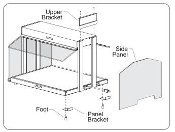
Figure 11. Installing the Side Panel
