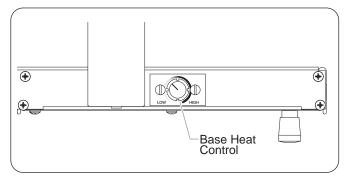
Figure 7. Base Controls for GRBW-XX Models
