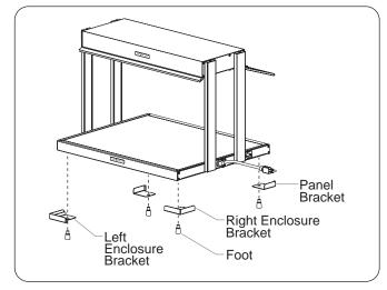
Figure 8. Installing the Brackets
