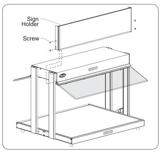
Figure 12. Display Sign Holder Assembly
