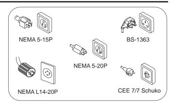
Figure 3. Plug Configurations
