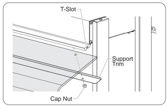
Figure 9. Installing the Front Enclosure
