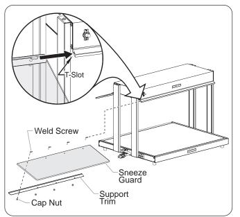
Figure 5. Installing the Sneeze Guard
