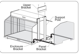
Figure 10. Installing the Front Enclosure and Side Panel
