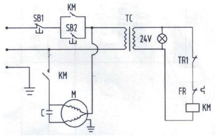
T--Motor C--Capacitor TC-Transformer SB1--Off Switch SB2--On Switch KM--Relay FR--Temperature limit TR1--Magnet Microswitch
