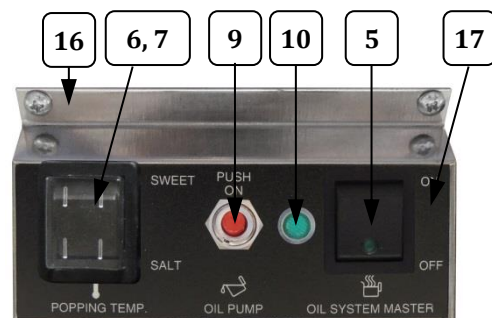
Switch Box for Back Counter Units with Oil Pump Switch and Salt-Sweet option
