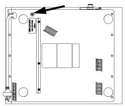
4. Using screwdriver; press down and turn the fuse holder cap to release it from the range.
