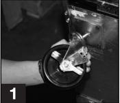
Thread castor into the underside of cabinet frame rail.
