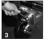
Use the tool provided to tighten the castor into place.
