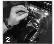
For leveling, insert the shim between the castor and frame rail.
