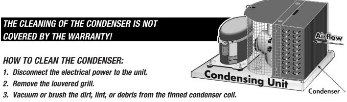
4. If you have a significant dirt build up you can blow out the condenser with compressed air. (CAUTION MUST BE USED to avoid eye injury. Eye protection is recommended.)
