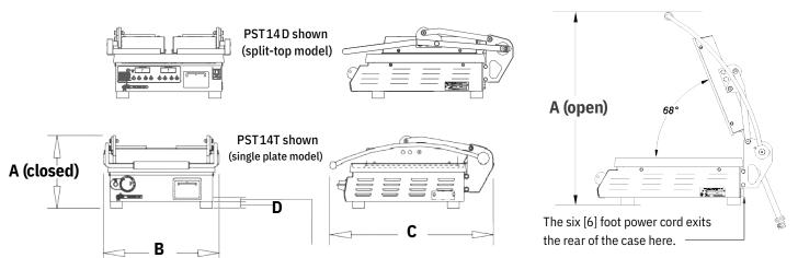
The cord exits approximately .625 in. (159 mm) up from the base of each model and from the right side [looking from the front] the cord is 1.5 in. (38 mm) from the side on the 7-in. model and 3.375 in. (86 mm) on the 14-in. model.
