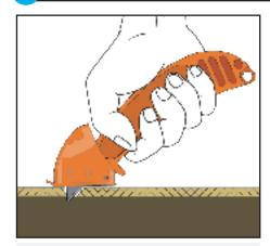
Firmly grasp the Lizard and press the blade guard down on cutting surface. The blade safety guard will retract allowing you to start your cut.
