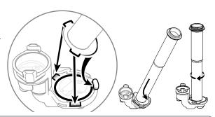
7 INSTALL MEDIUM O-RING onto discharge tube.
