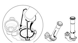
**INSTALL MEDIUM O-RING** onto discharge tube. Apply food equipment
