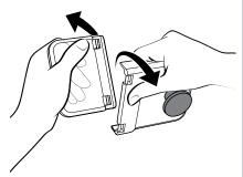
DISASSEMBLE Twist to snap hinges apart.
