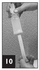
Push and remove the plunger through the bottom of the pump body.
