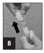
Place one hand over the elbow connector and spring. With the other hand, unscrew the pump body from the elbow connector.
