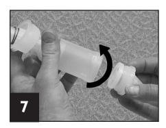
Unscrew and remove the pump bottom.
