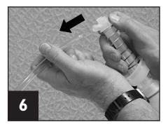
Gently twist and pull the end of the nozzle tube to remove.
