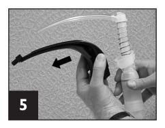
Slip the lower housing off the pump engine.
