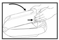
4. Close cover. **NOTE:** Pressure plate carriage will automatically release when cover is closed, applying pressure to napkins.
