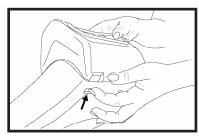
Locate 2 tabs under front of face and depress upward into base one at a time.
