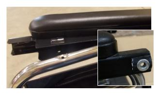
Remove arm pad and install bracket with jacknut installed as shown. Use one black washer on each long black screw to attach arm pad.
