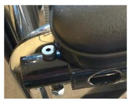
Install shoulder bolt and screw as shown.
