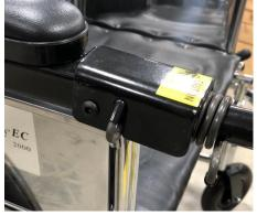
Slide spring and bracket over the rod on the right arm of the basket assembly. Attach the assembly to the bracket under the arm pad using the screw provided.
