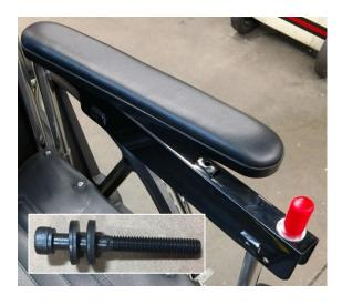
Remove left arm pad an install arm bracket under arm pad with rod facing up as shown. Use two black washers on each long black screw to attach arm pad.
