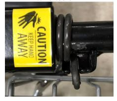
Continue to push tube in and align the end of the spring with the opening on the tab welded on the arm.
