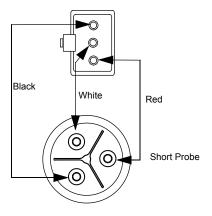
**Ohm water Level Probe and Wiring Harness**
