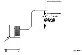
**35 ft. (10.7 m) Rise:** The maximum distance the Condenser or Condensing Unit can be above the ice machine.
