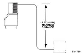
**15 ft. (4.5 m) Drop:** The maximum distance the Condenser or Condensing Unit can be below the ice machine.
