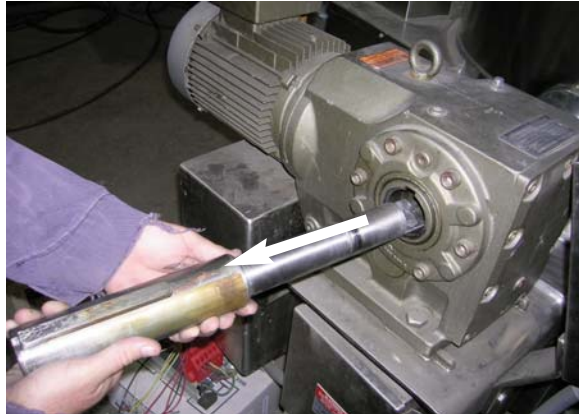
5. Gently hammer out shaft and remove.
