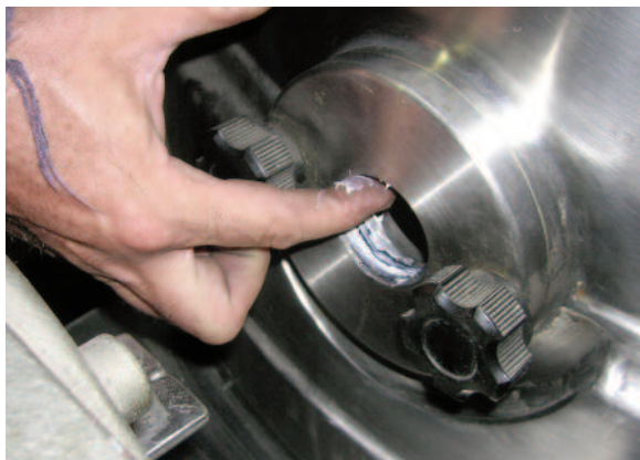
7. Grease seal with food grade grease.
