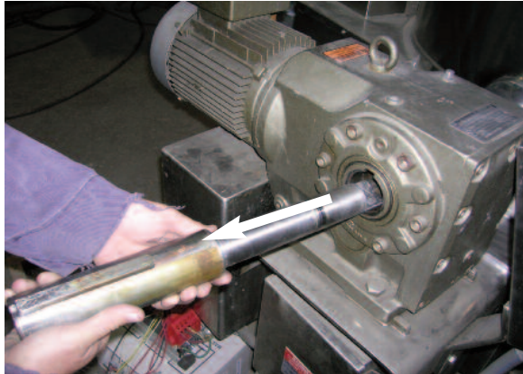
5. Gently hammer out shaft and remove.
