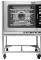
A high efficiency gas combustion chamber heats the cooking cavity in steam, combo and oven modes. All condensate exits through cavity drain. Oven/steam vent is provided. Safety or low water cutoff provided and reservoirs automatically drain when unit is turned off. Standing pilot with electronic ignition is standard.
