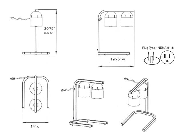
Electric: Attached 6-foot flexible, three-wire cord with ground plug (NEMA 5-15). Construction: Aluminum Finish: Brushed aluminum On/Off Switch: Easy-to-use and access
