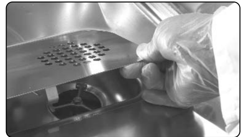
Remove and rinse drain trough with hand shower
