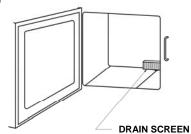
Figure 2-4 Compartment Drain Screen
