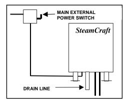
Figure 2-1 Main External Power Switch
