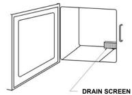
Figure 2-4 Compartment Drain Screen
