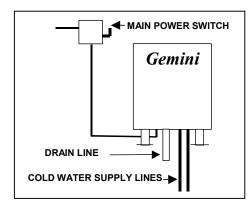
Figure 6-2 External Main Power Switch
