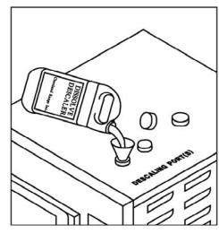
Figure 6-1 Descaling Port
