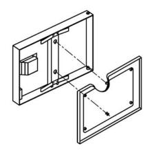
Figure 5-1 Door Gasket Assembly
