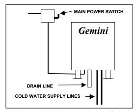
Figure 2-1 Main External Power Switch
