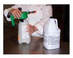
**STEP 2** Fill the spray bottle with a mild oven detergent. We recommend the following cleaners: Greasecutter Plus by Ecolab, EZ Clean by Cello, or Advance Oven Cleaner by Diversey-Lever. **DO NOT USE ABRASIVE CLEANERS ON YOUR BLODGETT COMBI.** Be sure to read and follow the MSDS or safety instructions on the bottle of your oven cleaner.
