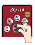
**STEP 6** With the oven door open, turn the oven to the OFF mode. The remainder of the process is automatic. The delime lamp stays lit until deliming is completed.
