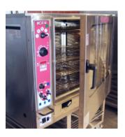
STEP 7 Leave the door open overnight to vent the oven. If the oven will not be used for an extended period of time, place the oven in hot air mode to dry.
