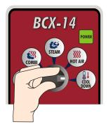
STEP 1 Open the oven door. Place the oven in cool down mode. Let the oven cool to below 140°F (60°C).
