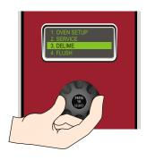
step 6 Turn the dial to highlight DELIME. Press the center of the dial to select.
