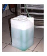
STEP 3 Fill the deliming fluid container. Use a non-diluted deliming agent such as *Lime Away* by Eco-Labs or *Lime Out* by US Chemical. Be sure to read and follow the MSDS or safety instructions on the bottle of your deliming agent.
