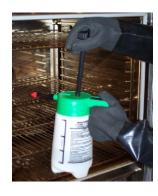
STEP 3 Pump the bottle twenty times to build up pressure. The higher the pressure, the finer the spray.
