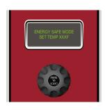
STEP 9 When the deliming process is complete, the control enters the energy safe mode. The oven can now be used normally.
