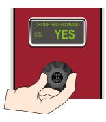
STEP 8 Turn the dial to highlight YES, this confirms that you want to begin the deliming process. Press the center of the dial to select. The remainder of the process is automatic. The display counts down the fill and delime time remaining.
