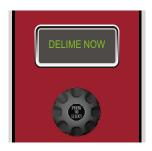
STEP 1 When it is time to delime your BCX, the display reads DELIME NOW. Press the Escape key to clear the display. The message will return until the unit is delimed. This is a warning only, the oven can be used all day before deliming.
