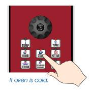
**STEP 2** The boiler should be warm to delime. If the oven is hot, place in the cool down mode with the door open until the cavity is below 140°F (60°C).
