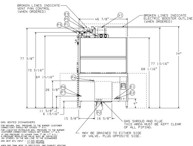
WHEN GAS TANK HEAT IS SPECIFIED, GAS EXHAUST VENTING MUST BE INSTALLED ACCORDING TO LOCAL CODE: DO NOT CONNECT FLUE TO POWER VENT.
